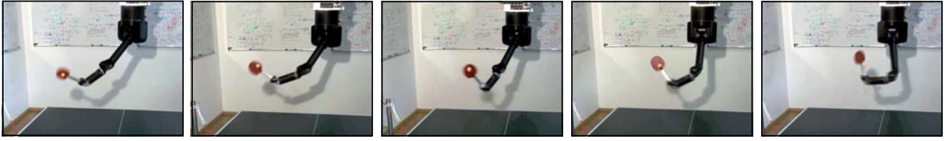
Figure 3.7: Generalization to various targets (five different forehands at posture ③) are shown approximately when hitting the ball.
