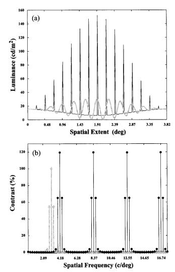
Fig. 2. (a) Cross-sectional luminance profile of a 4.18-c/deg pulse train along a vertical slice through the center of the spatial Hanning window. Luminance  $(cd/m^2)$  is plotted as a function of distance (degrees of visual angle). A sinusoidal grating of the same mean luminance, 100% contrast, and slightly lower spatial frequency is shown for comparison. (b) Contrast spectrum of the pulse-train and sinusoidal gratings of (a) as a function of spatial frequency.
