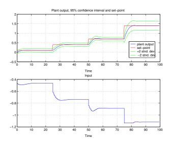
Fig. 3. Constrained case ( $\sigma_{max}=0.13$ ): response of GP model based control (upper figure) and control signal (bottom figure)
