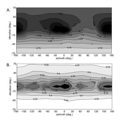
Figure 3: Distance statistics of an indoor robot (0 azimuth corresponds to forward direction; the distances on the contour lines are given in m): A. Average distances from the origin in the visual field (N = 26). Darker areas represent larger distances. B. Distance standard deviation in the visual field (N = 26). Darker areas represent stronger deviations.
