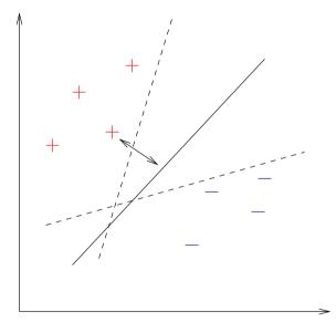
Maximize the margin  $\rightarrow$  leads to 'robust' solution  $\rightarrow$  Support Vector Machines
