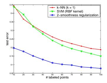
Digit recognition with USPS handwritten 16x16 digits dataset for a total of 9298. The left panel shows test errors for different algorithms with the number of labeled points increasing from 10 to 100.
